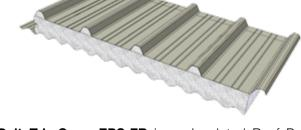
DeltaTrimCorro-EPS-FR is an Insulated Roof Panel System, comprising of two pre-painted, roll-formed steel skins, bonded to a fire retardant grade expanded polystyrene insulating core.
